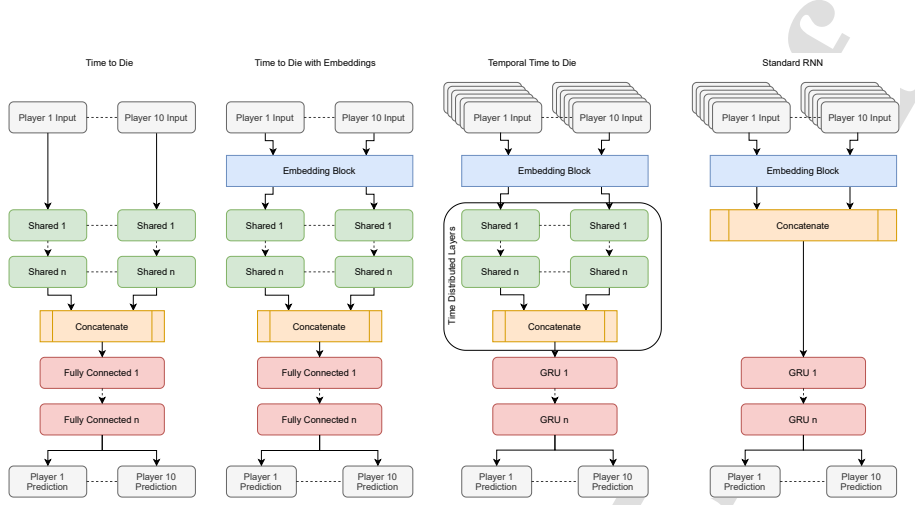
Figure 2: Architectures for each model presented in the paper. First, the standard Time to Die model used in TtD_A and TtD_B . Second, incorporating embeddings into the model used in TtD_+ and TtD_2 (for an explanation of the embedding block see Figure 3). Third, the Temporal Time to Die model TtD_{temp} . Fourth, a temporal model which just uses RNN layers called StandardRNN .
